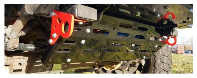
Offer up the guard to the two side plates and recovery points and loosely bolt together using the M8 button head Allen bolts, nuts and washers.
