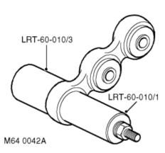
4. Use LRT-60-010/1 and LRT-60-010/3 to press bushes from transverse links and pivot housing.
