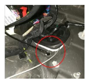
Run the power cables into the cabin via this hole.
