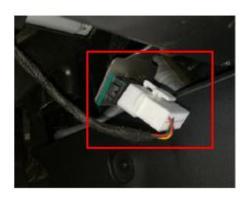
Locate the OBD connector in the foot well and connect the plug from the wiring loom.
