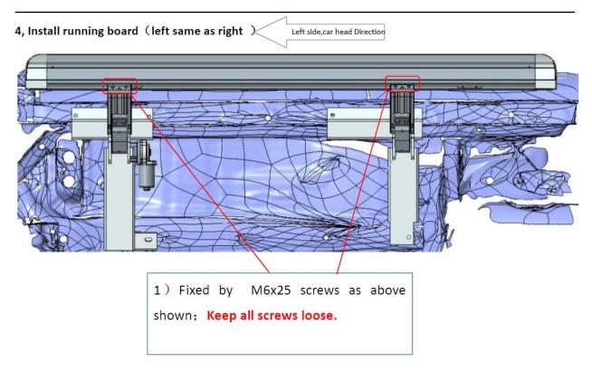
All fixings should be left loose so the position and level of the side steps can be adjusted against the body line of the car.
