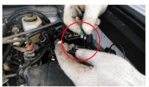
Remove the fuse. This is so the steps do not operate until you are ready.
