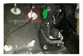
The negative / earth wire should be run to this body earth point above the brake pedal.
