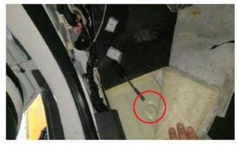
Remove the trim from around the front N/S door, pull back the carpet to revel this hole, the motor wires can be passed up through this hole. Repeat on the O/S for the wires from the motors on the other side.
