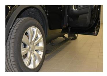
Ensure both front and rear doors operate the step on that side.
