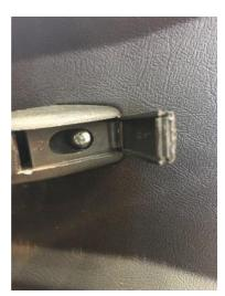
6. Remove the two trim clips at the corners of the door card:
