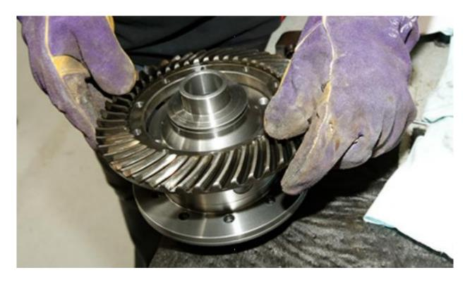
Position the crown wheel onto the E Locker center.
