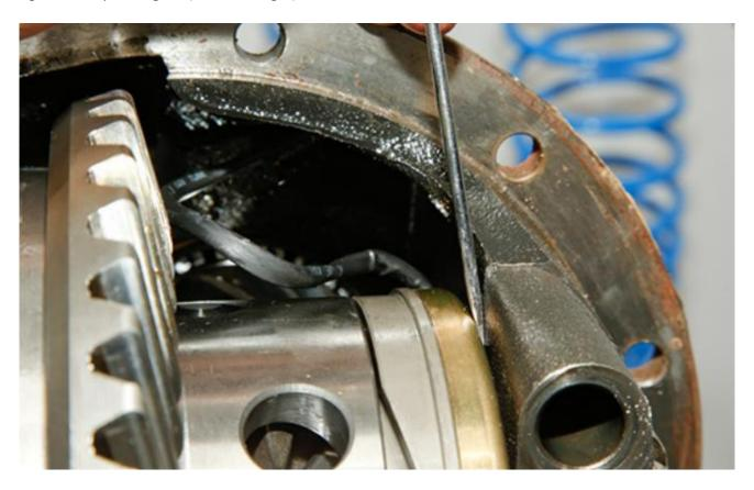
Position the electric cable and anti-rotation peg on the electromagnet to the top so they are visible when you fit the bearing caps.
