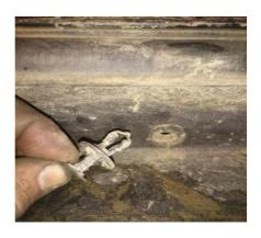
3. Remove the 10mm nut from the centre of the lower section at the rear of the front wing; the plastic trim should now be free to be removed. Trim off the excess thread from front wing mounting bolt.
