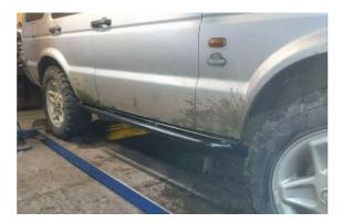
NOTE\* The rear most hole in the Rockslider is not used.
