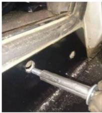
7. When fitting the crush tubes from the inner, nearest the chassis side the bolt need to come through the hole from the outside and then the tube slid into the hole and over the bolt.
