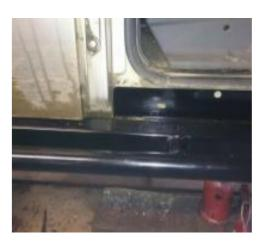
5. When you are happy with the positioning of the Rockslider mark and drill the holes, the round holes need to be drilled to 13mm (5 holes inner, nearest side to chassis, 4 holes on the outside) to allow the crush tubes to be inserted.
