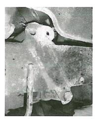
Fit the new chassis plate as shown below. Place two of the large M12 washers over the bolts and use as spacers between the plate and chassis. Without these spacers the plate will interfere with the tie down point.
