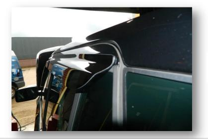
Rear deflectors should align perfectly with the door frame.
