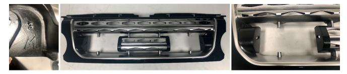
After checking remove the mounts, using the shorter bolts and washers where required bolt the correct mount to each side of the light, slide the light and mount onto the centre part of the grill first and then onto the outer part.
