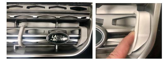
Check and double check that you are happy with the fit of the cutting guides, a hack saw blade is best to cut the grill.
