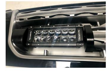
When you are happy with the fit, drill the hole through the grill to line up with the hole in the outer mount and use the supplied screw to secure. Do not over tighten.
