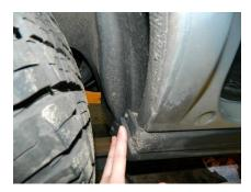
2. Remove the 7 trim clips on underside of standard side sill trim.
