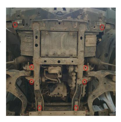
Leave bolts loose to allow you to centralise the guard and position it fully front to back. When happy tighten the guard
