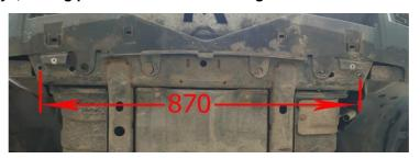
Lying on your back, attach the chassis plates with the bottom of the 'L' brackets facing rearwards. Using the M8 bolts, place bolts into the holes in the bumper support. Use washers on the bolt head and between the bracket and the Nyloc nut.
