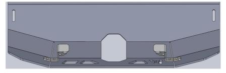
Attach striker brackets to the main guard with M8 Button head bolts
