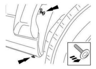
3. Fit the clips to the brackets, fit the clips to the car and then attach the brackets to the car –
