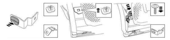
4. Hold the mud flap in position and then replace the 3 trim clips securing the mud flap as shown –
